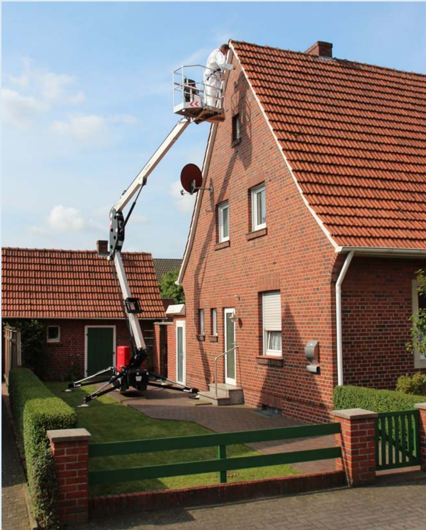
The light LEO15GT can be towed on standard trailers. With the cable remote control loading is quick and easy.
