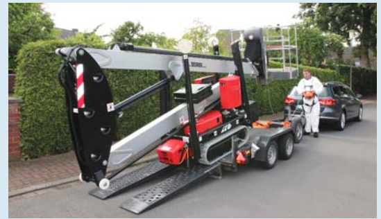
The light LEO15GT can be towed on standard trailers. With the cable remote control loading is quick and easy.
