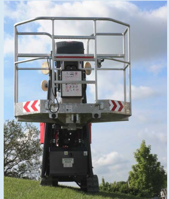
The optional adjustable track chassis allows driving safely alongside slopes and to increase ground clearance for better terrainability.
