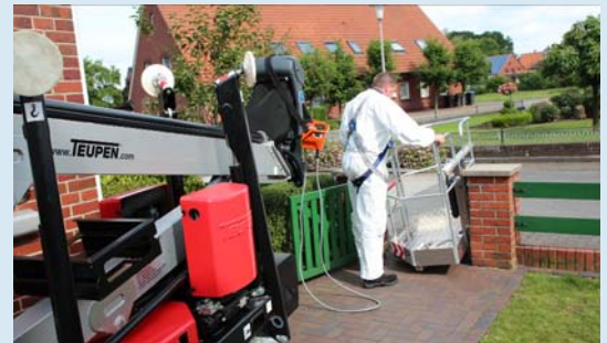
For passing narrow entrances the basket is easily detachable - mounted rollers make moving it around easy.
