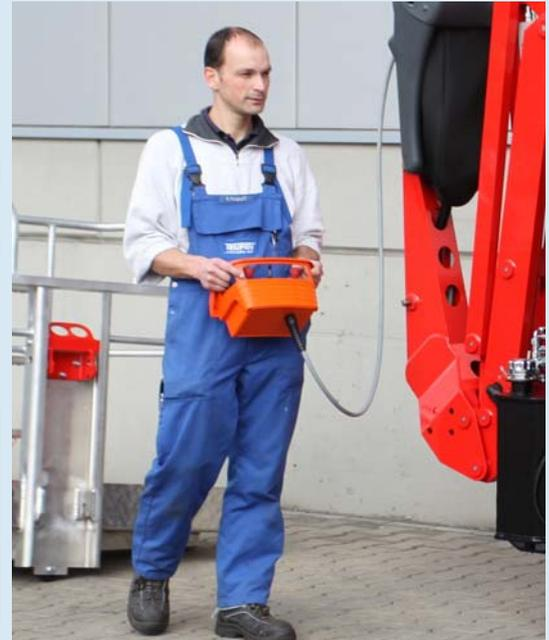
The cable remote control gives the operator a better overview when driving and setting up the lift.
