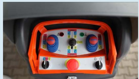
Teupen controls are well-arranged with color coded functions. Only two joysticks and one switch for the entire lift operation.
