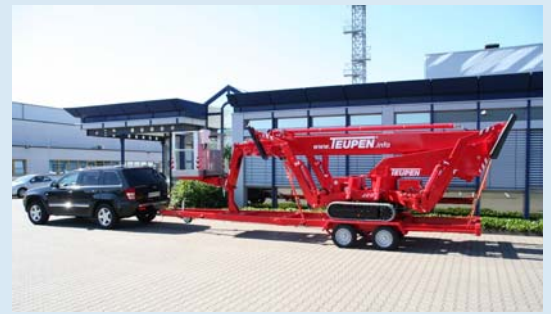
For easy transport the LE25T is easily towed on standard trailer. Customized trailers are also available.
