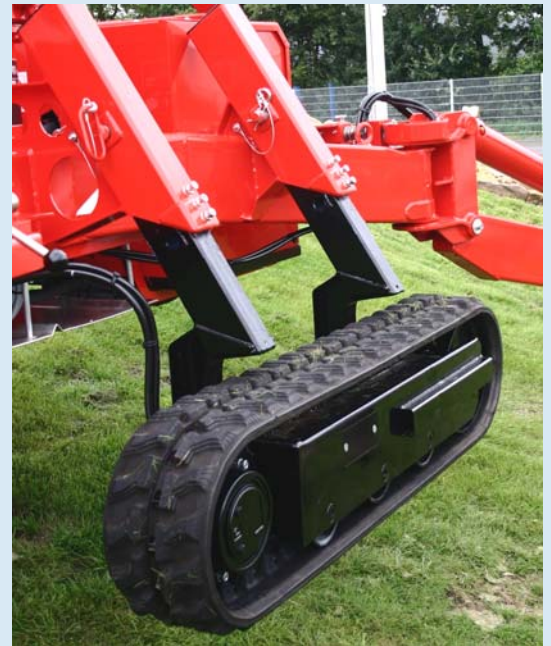
The mechanically height- and width adjustable track chassis provides more ground clearance and makes the lift more versatile for ultimate performance in rough terrain.
