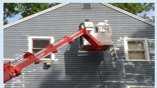
The LE25T features a 180° rotatable basket for more versatility when positioning the basket into tight spots, working alongside facades or in trees.
