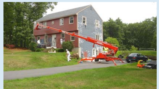
In the robust stabilisers several safety systems constantly monitor all setup functions and the ground pressure directly in the stabiliser plate.
