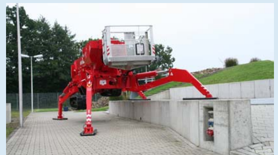
The multi-level, multi-position automatic levelling system reliably sets up the machine - also in uneven terrain or in confined work areas.
