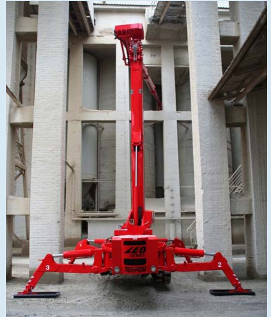
In the robust stabilisers several safety systems constantly monitor all setup functions and the ground pressure directly in the stabiliser plate.
