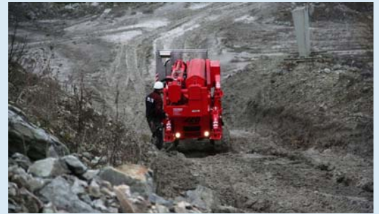
On the powerful track drive the LE40GTX can be manoeuvred precisely. It even allows the machine climb steep slopes, stairs and drive with ease in rough terrain.
