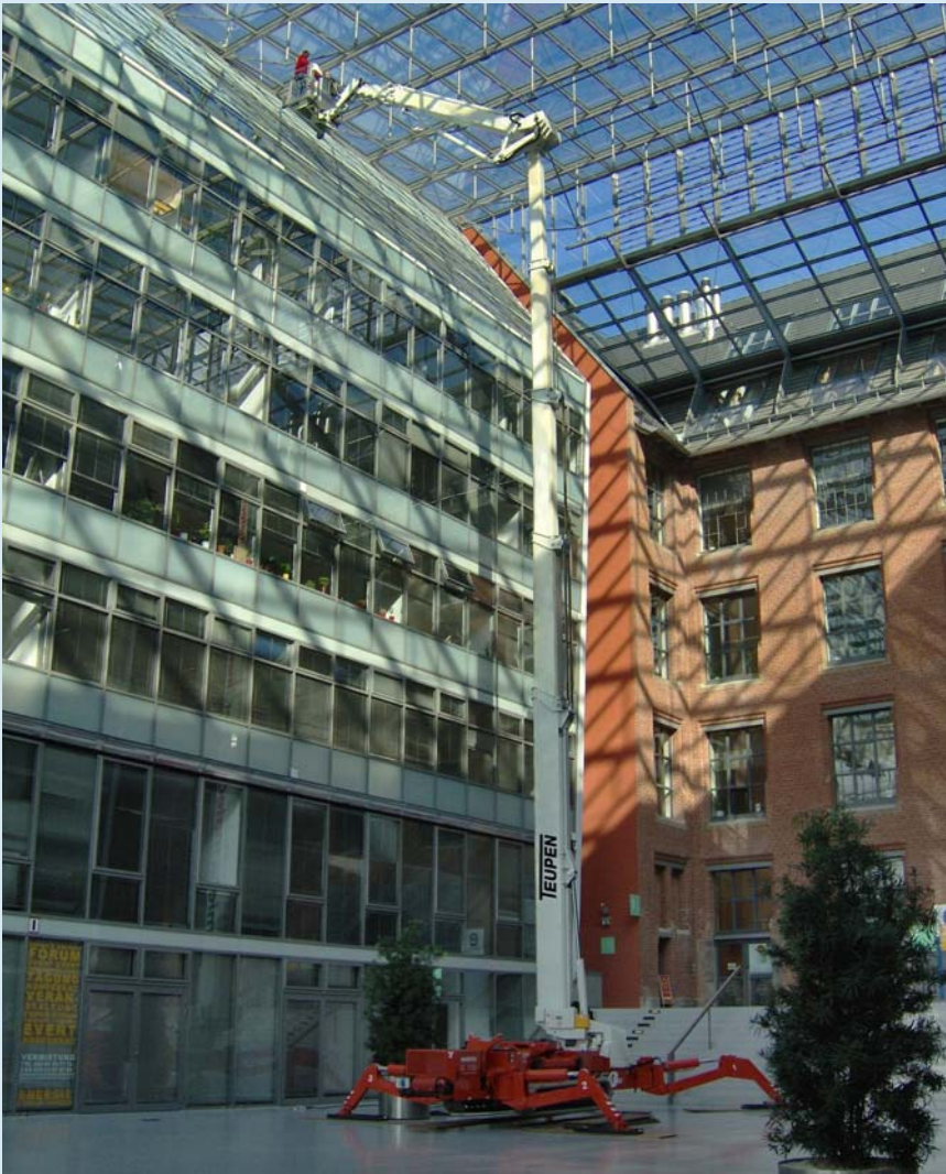
On the powerful track drive the LE050GTX can be manoeuvred on delicate floor types as well as in rough terrain. It even allows the machine climb steep slopes and stairs.
